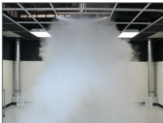
Throw test in laboratory mock-up room
