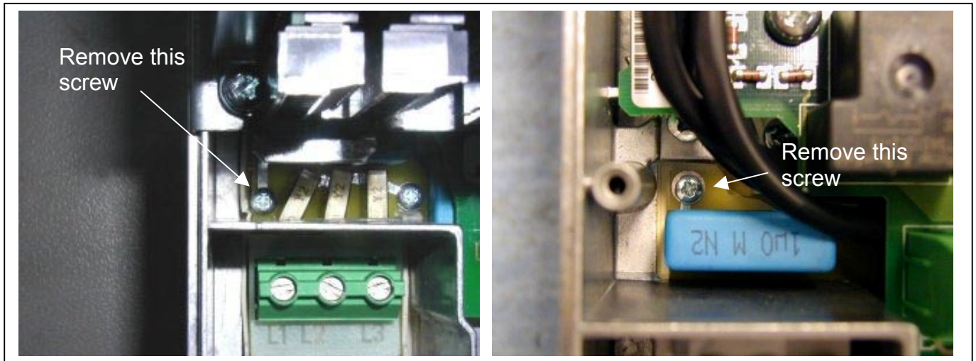
Figure 5-13. Changing of EMC protection class, FR4 (left) and FR5 (right).
